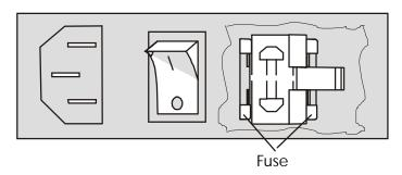
Figure 5-1: AC Fuse Replacement
